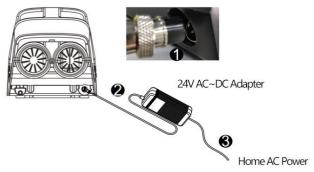
① Air conditioning power connectors  $\Rightarrow$  ② Power adapters  $\Rightarrow$  ③ Home AC 100-240V (50-60Hz)
